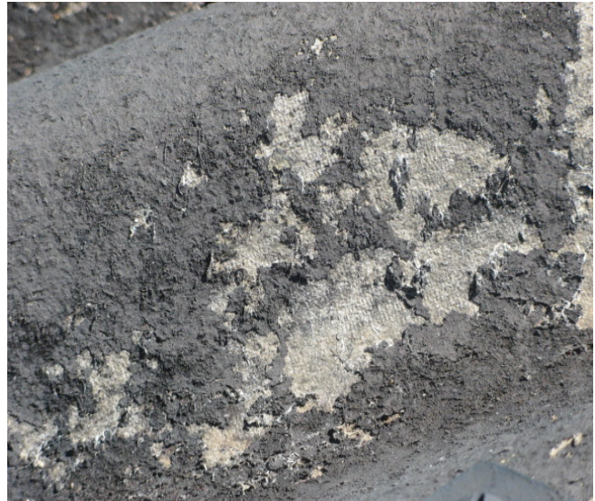
Photo 4. Surface flaking from weathering
